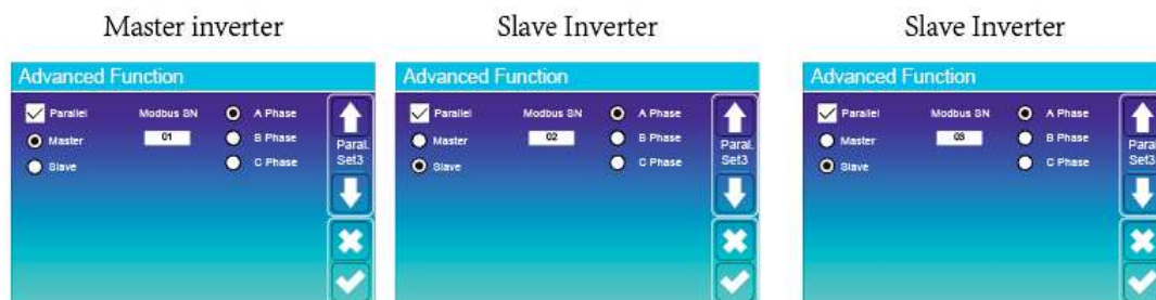
Single phase Interface configurations
